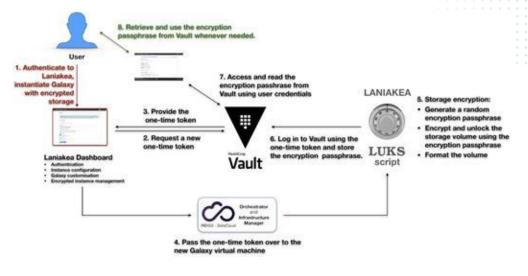
The encryption layer sits between the physical disk and the file system. Galaxy, or any other software is unaware of storage encryption, exploiting a specific mount point in order to store and retrieve files. A short lived token, usable only once, is delivered to the encryption script on the VM. The Storage volume is encrypted and the passphrase is sent to Vault. After the instance has been successfully deployed the user can retrieve his password through the Dashboard.
