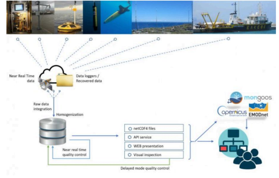
The POSEIDON monitoring network consists of a series of different platform types recording in situ data in the vicinity of the Greek seas:
